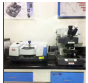
Nicolet iS50 Fourier Transform Infrared Spectrometer (FTIR) Spectral Range: 350-7800 1/cm-1
